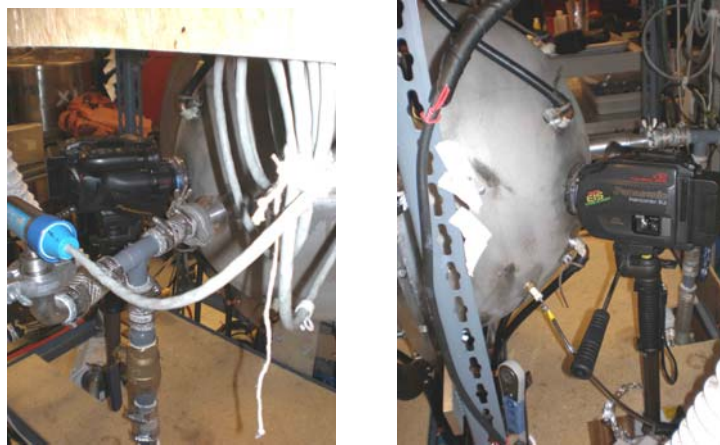
Figure 3.21: First camera mount on monopod (minus Faraday cage) showing early plumbing
