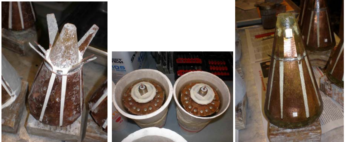
Figure 4.5: Stripping off ceramic; casting in solid epoxy; finished before BN paint (note the O-ring flanges covered by masking tape)
