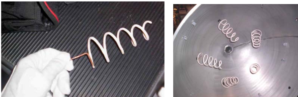
Figure 3.13: Early antenna design, before and after mounting in hemisphere (2006)
