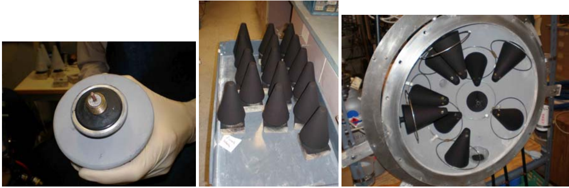
Figure 5.1: O-ring seal with Q putty; painting the antennas; mounted on South Hemisphere
