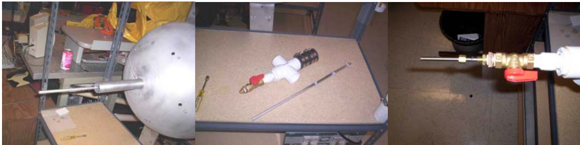
Figure 3.22: Mounting for sparker, allowing entrance through South hemisphere polar pipe
