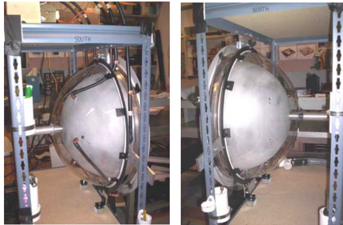
Figure 3.14: Acrylic magnet spindles; never wound the wire on them
