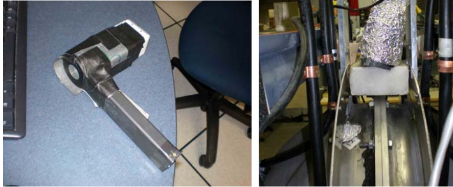
Figure 4.6: Scintillator detector with camera, and mounted on reactor with paraffin
