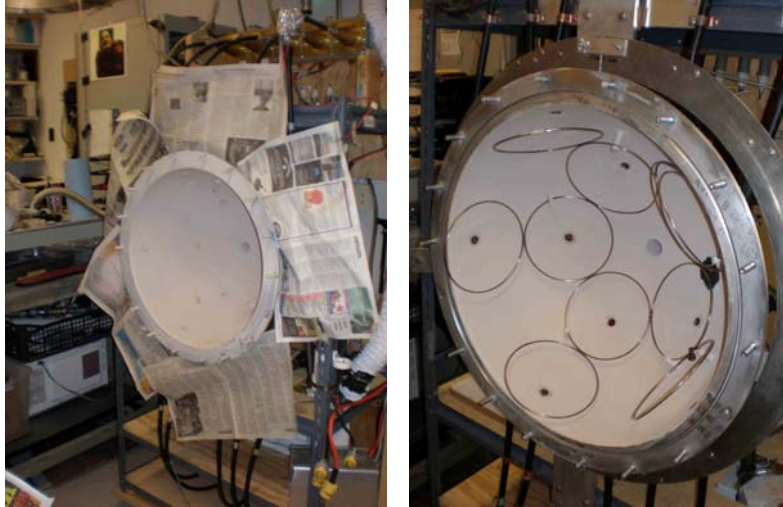
Figure 3.26: water-based ceramic spray job; final grid installed
