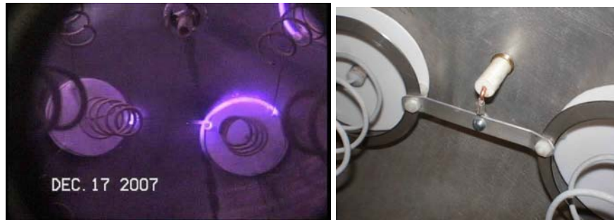
Figure 3.25: thin wire in operation; replacement with sheet stainless circles
